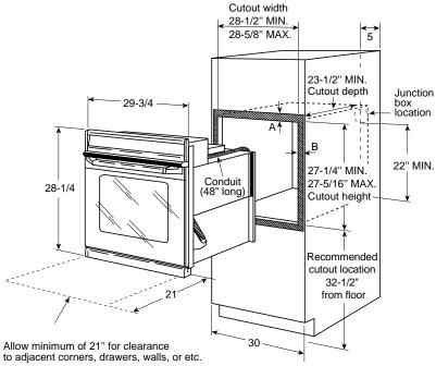
A=Allow 1" overlap of oven over top and bottom edges of cutout. B=Allow 11/16"-3/4" for overlap of oven over side edges of cutout.
